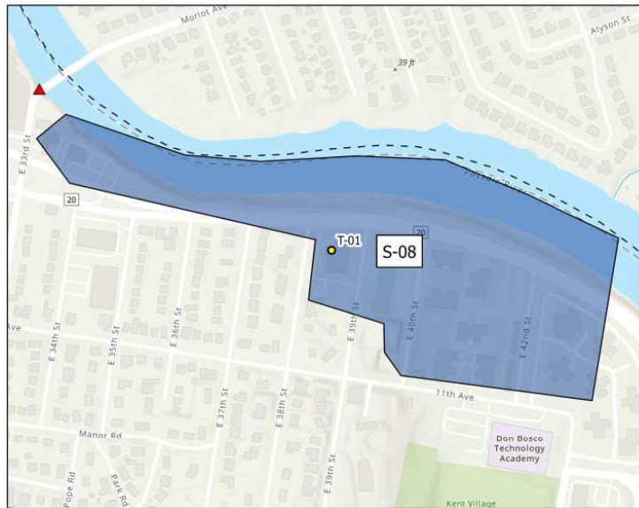
Figure 23: Sewershed S-08, Site IDs, and CSO Outfall
